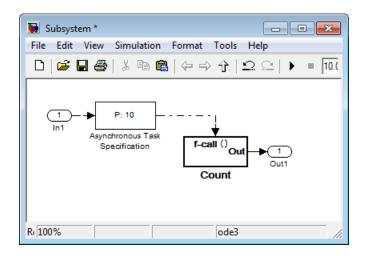
Whereas, if the priority of the Asynchronous Task Specification block is set to the empty matrix, [], the priority of the Async Interrupt can be a value other than 10.
